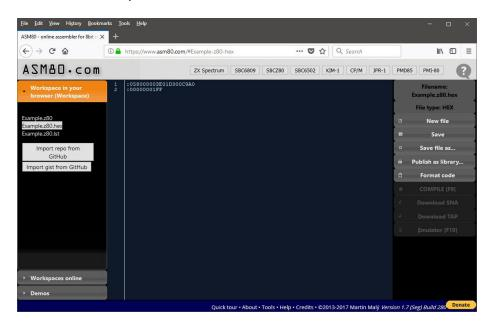
The hex file contains the machine code program bytes in Intel Hex format. This is a commonly used format for storing and transferring machine code programs. It can be opened by most EPROM programmers and can also be sent directly to the Small Computer Monitor.
