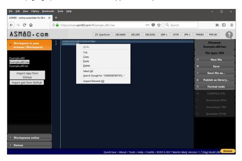
We now have the Intel Hex file text on the clipboard ready to transfer to the target RC2014 system via a terminal program.
